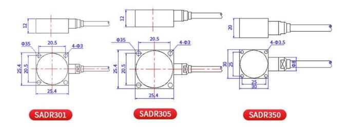
The SADR series capacitive accelerometers utilize a differential capacitive sensing element, whose output voltage depends on the tilt angle relative to gravity. The sensor's tilt angle output is determined by the magnitude of gravity parallel to the sensor. This principle is employed to measure the tilt angle. When measuring angles greater than 10°, the following formula should be used for calculation:
