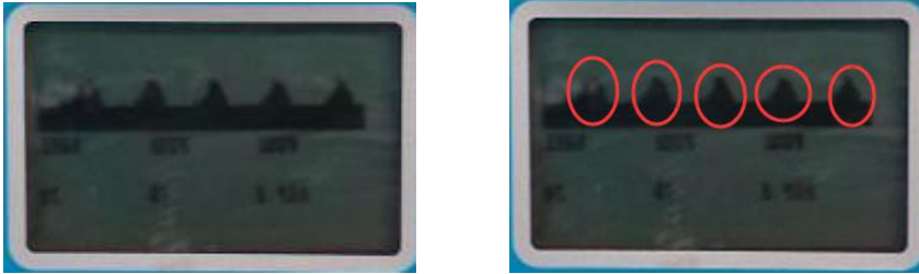
Fig. 7 Echo Pattern under Interference of Frequency Converter
