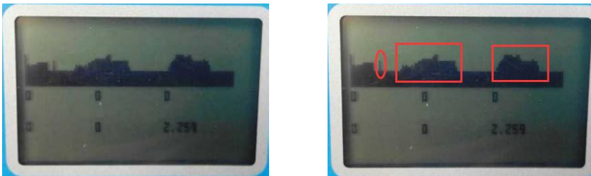
Fig. 8 Echo Pattern under Interference of Frequency Converter
