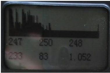
Fig. 4 Echo Pattern after Probe Lifting
