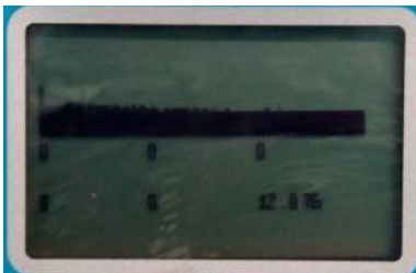
Fig. 6 Echo Pattern under Electromagnetic Interference
