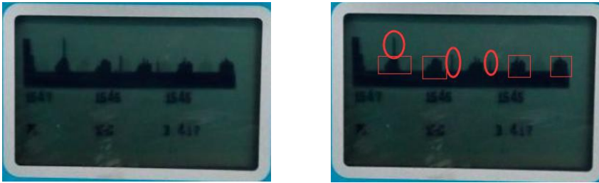
Fig. 9 Echo Pattern under Interference of Frequency Converter
