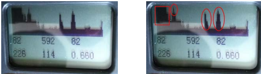
Fig. 3 Echo Pattern after Liquid Enters Blind Area
