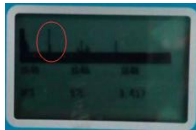
Fig. 5 Normal Echoed Signals
