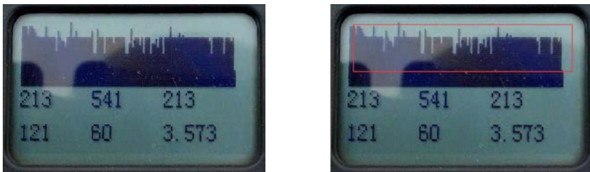
Fig. 10 Echo Pattern under Strong Interference
