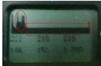
Fig. 12 Echo when Probe is Out of Connecting Pipe
